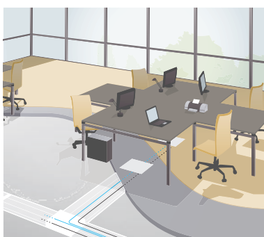
Screed floor system
