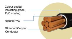
"HAVELLS" manufacturing and supply premium quality multi core flexible cables with copper conductor for various industrial and domestic applications where portable, movable equipment or flexibility make installation easier, Special formulated "Polyvinyl Chloride" (PVC) used for insulation and sheath tends to flexibility of cables.
